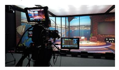
"Aquilon is so versatile and powerful that it can be adapted to any project, so we decided to include it in the new studio from the beginning," Fonseca says. The XR studio features a 14-meter, curved 2mm LED videowall and 4mm LED floor, a media server to facilitate XR workflow, two 3D game engines, one fixed and two tracked cameras, a 2.8mm LED comfort monitor and several 55-inch monitors.
