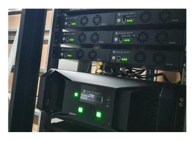
DPH104 is a high-performance latency-free 4K image processor able to convert one 4K DisplayPort output from a LivePremier™ presentation system, such as Aquilon C, or a Picturall Mark II media server to four independent 1080p HDMI outputs. All the outputs on the DPH104 can be used with native resolution just like they were directly connected to the source system. DPH104 does not require software or configuration and guarantees an easy and trouble-free installation experience.
