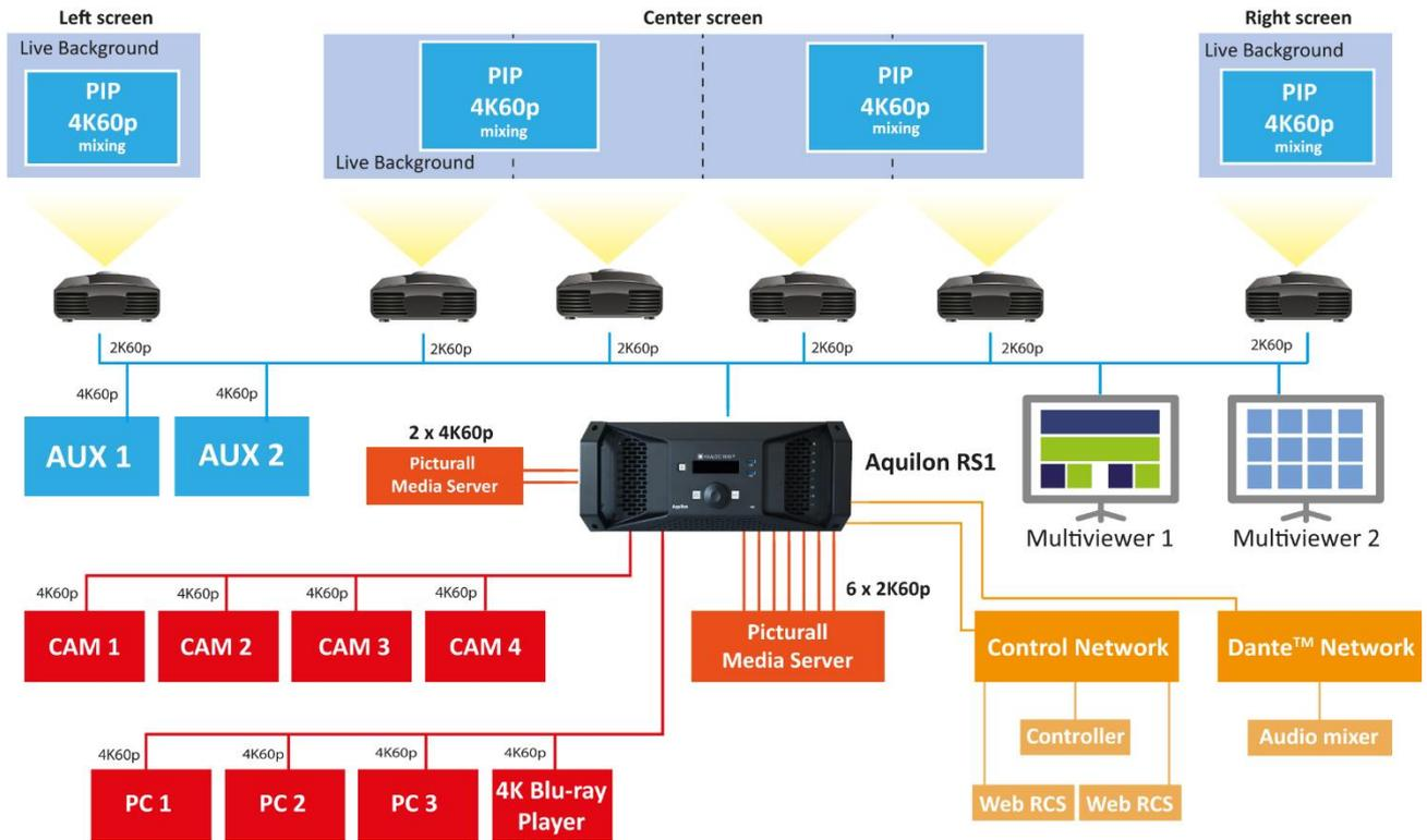
**Aquilon RS1 can drive one 8K60p LED walls and 4x 4K60p AUX outputs**
