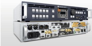
**VIO 4K (Ref. V701)** is a powerful multi-format converter offering the latest generation of digital connectivity. Natively equipped with 7 inputs and 1 multi-plug output, **VIO 4K** enables the conversion of a multitude of signals including: Dual-link DVI, DisplayPort, HDMI, 3G-SDI, SPF module cage, and universal analog, into an impressive array of output signal formats up to 4K 30Hz (4K 60Hz can be accomplished via expansion modules).
