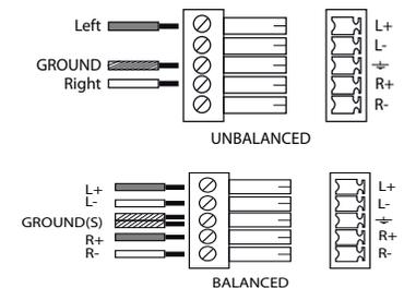
Outputs #1 to #2: Balanced & unbalanced connection
