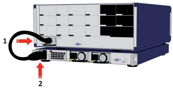
The second step is to insert the head frame into the **LiveCore™** device and connect the **SpeakON™** connector to the **Secure Power Unit**.
