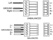
Outputs #1 to #2: Balanced & unbalanced connection
