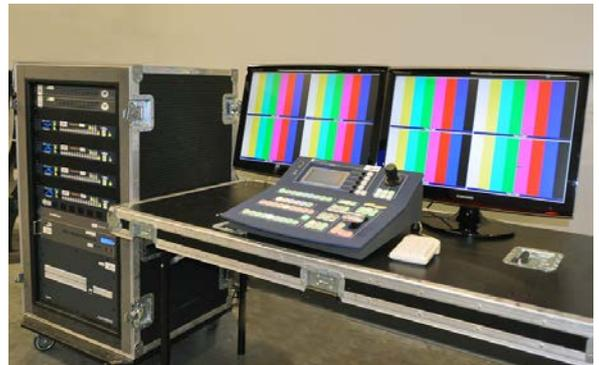
**Pulse** is a Multi-Layer Mixer Scaler Seamless Switcher with full digital in/out processing plus universal analog inputs. It offers 10 direct inputs including 2 fitted with DVI and 2 fitted with 3G-SDI. **Orchestra** is a powerful, intuitive and ergonomic Remote Controller designed to manage independently or simultaneously a variety of **Analog Way's** Switchers as well as a variety of up-stream matrix devices.
