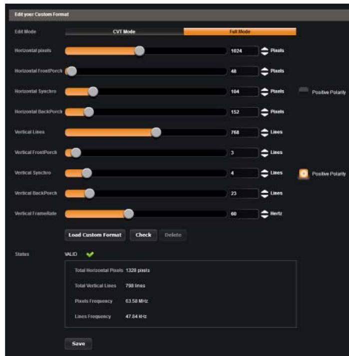
Once the parameters are set, they must be checked to verify that they are compatible with the device capabilities.
