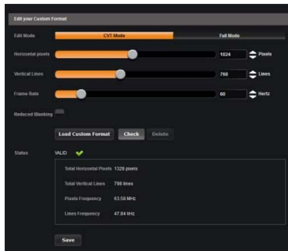
Once the parameters are set, they must be checked to verify that they are compliant with the CVT standard and if they are compatible with the device capabilities.
