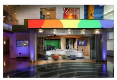
The studio entrance is topped by a ribbon-shaped Planar LED video display with a resolution of 5120 x 360. Analog Way's Picturall Quad media server enables full-screen playback of custom content across the display at full resolution.
