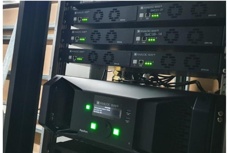
DPH104 is a high-performance latency-free 4K image processor able to convert one 4K DisplayPort output from a LivePremier™ presentation system, such as Aquilon C, or a Picturall Mark II media server to four independent 1080p HDMI outputs. All the outputs on the DPH104 can be used with native resolution just like they were directly connected to the source system. DPH104 does not require software or configuration and guarantees an easy and trouble-free installation experience.
